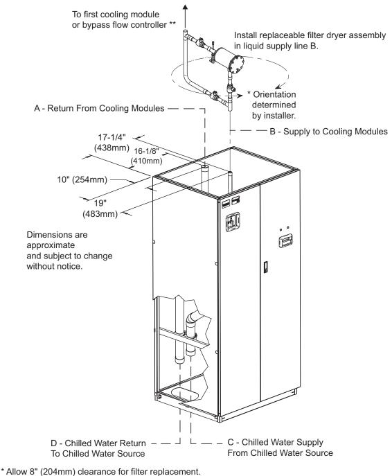
\*\* To ensure ensure all refrigerant flow is filtered, install the filter dryer assembly between the discharge line of the Liebert XDP and the first bypass flow controller or the first cooling module. DPN000767 Pg. 3, Rev. 6
